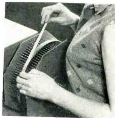
Securing filled reel by pressing down 12-inch trailing leader
