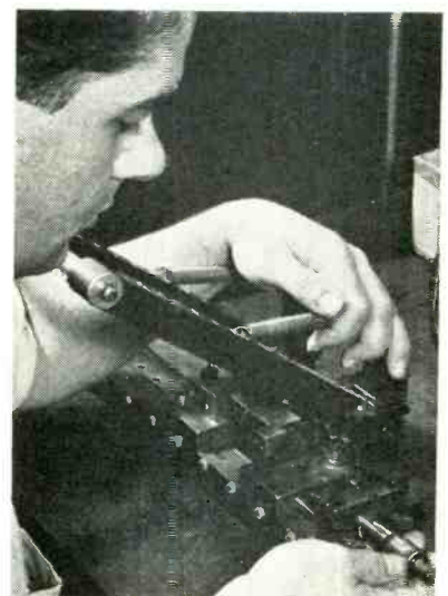
Adjusting micrometer to set right-hand anvil-blade combination to desired thousandth of inch
