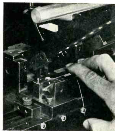
Placing resistor card in position on cutting anvils. Hole in left end of card, fitting over positioning peg, is cut off along with surplus length at other end of card
