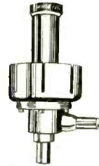
WATER-COOLED—STYLE WC5 • For high-frequency, high-power TV, FM, low-reactance uses. Allows mounting on 3" coax line with both water intake and outlet at RF ground potential. Interchangeable resistance elements.
