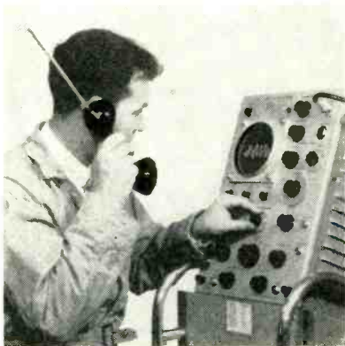
Technician tests output of voice-powered radio transmitter by watching waveforms of his voice on cathode-ray oscilloscope
