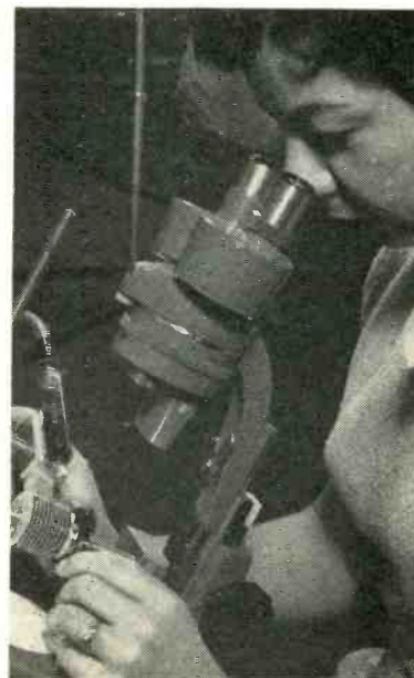
Anchoring turns of precision pot in core with varnish applied by hypo under air pressure
