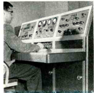
MONITOR CONSOLE —Main lamps come on only to indicate malfunctions. Emergency button stops all machines
