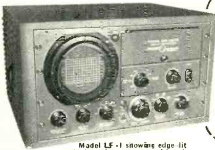
Model LP-1 showing edge-lit reticule and camera mount bezel.
