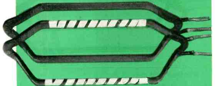
Two form wound coils for a Fairbanks-Morse 4160 volt Alternator. Lower coil has end sections insulated with "Natvar 400" extruded tape. Slot section is wound with a sacrifice tape, which is later removed and entire coil is wound with linen tape. Upper view of coil shows completed form, after final varnish dip and bake, ready for insertion in stator.
