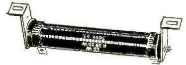
HIGH-POWER—STYLE R • 25 to 1,000,000 ohms; ratings from 7- to 115-watts; noninductive. Standard tolerance \pm 2\% 10 to 1,000,000 ohms. Exceptionally good noise and frequency characteristics. Superior moisture resistance and overload capacity.
