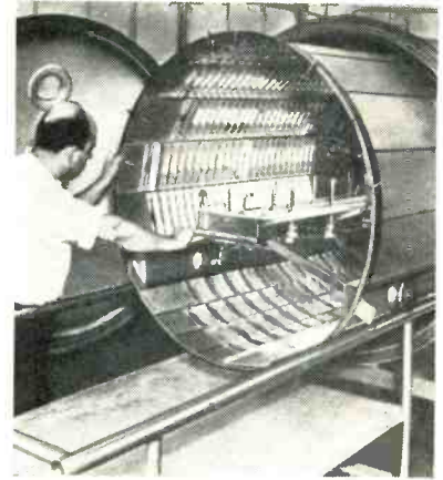
Type of metallizing unit used for depositing selenium. Drum rolls out on pipe rails for loading
