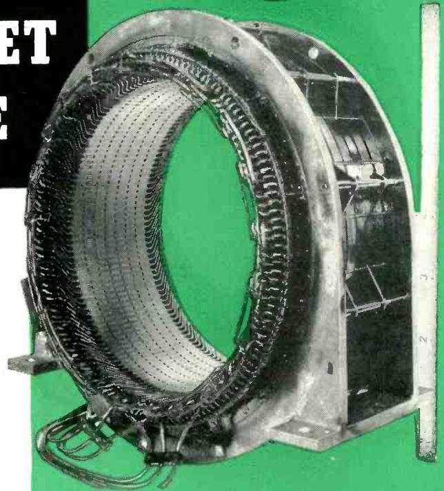
Stator showing open slot construction of the Fairbanks-Morse Type TGZO Alternator, 1405 kva — 300 r.p.m. — 3 phase — 60 cycle — 2400/4160 volts — 80% p.f. — for direct connection to a diesel or dual-fuel engine, for utility, municipal and industrial power generation. Since they are frequently subjected to prolonged overloads in this type of service, they are designed for 50°C temperature rise above 40°C ambient. Coils, insulated and protected with "Natvar 400" extruded tape are tested at 9520 volts for one minute.
