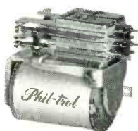
TYPE 4BQA — Miniature multi-contact relay; high speed, sensitive, available with printed circuit or taper tabs. O.D. 1-11/16" L x 1 1/8" W
